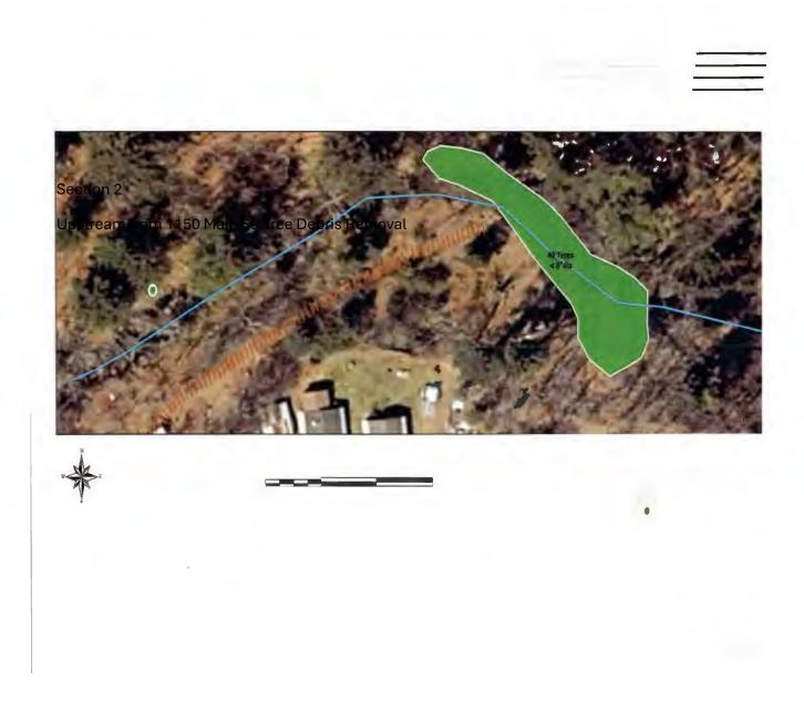
Green Areas indicate deposits of Tree Debris to be removed, chipped, and hauled to disposal site by CONTRACTOR.
